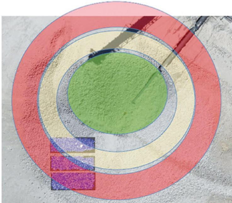
ing can be used to improve performance is with the material size in the 'red zone' as seen in the image (below): now, when an operation wants to start pushing outside material through the process, workers can optimise kiln settings based on the image-analysis data collected.
